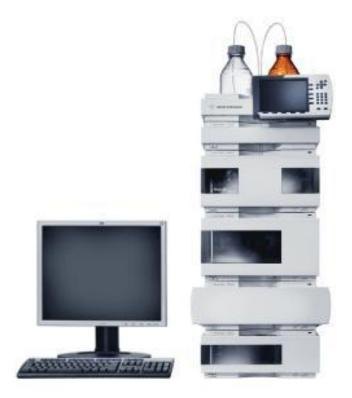
**Figure 1-7 Advanced HPLC instrument**
